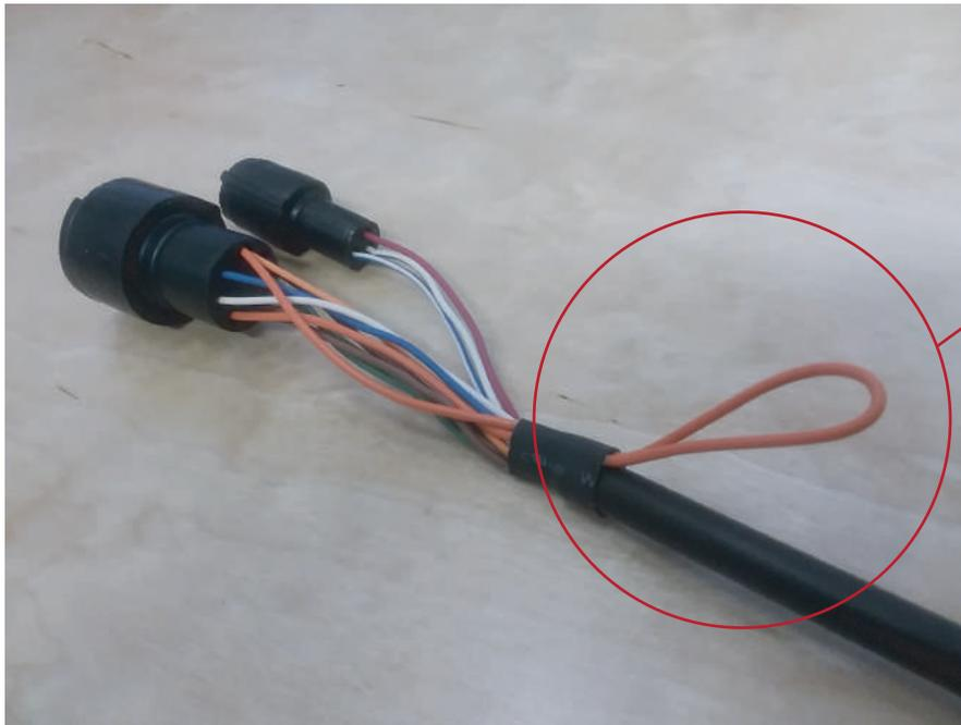
The photo above shows the Hiniker Vee Blade control harness. It was designed with access (the loop) to the Orange lighting trigger wire for operators who prefer a headlight switch. All other Hiniker control harnesses and the Meyer 12-Pin control harnesses have this same orange wire lighting loop.
